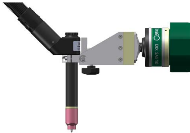
Torch head in folded position to replace the tungsten electrode.
