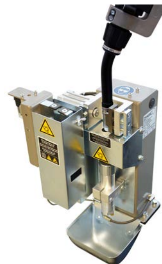
Robot with mounted DINSE torch head during the cleaning in the torch cleaning station
